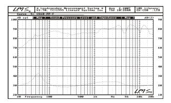
TECHNICAL DATA ARE MEASURED WITH LMS-EQUIPMENT ACCORDING EN-60268-5.
